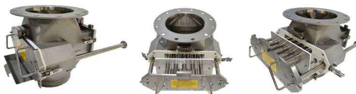
This equipment is manufactured with rare-earth magnetic material, tested and certified to 12000 Gauss on the contact surface. It has powerful magnetic forces and is commonly used in the food and pharmaceutical industries.
