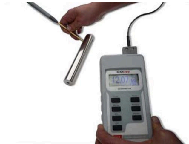
The Magnetic Tube being tested to 12000 gauss
