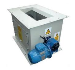
High intensity (3500 gauss) Rare Earth Housed Magnetic Drum 300 dia  $\times$  600 long for metal contamination removal in a mineral plant in a high temperature environment. The motor was IP 65 rated, tropicalised with anti condensation heaters, and fitted with motion sensors.
