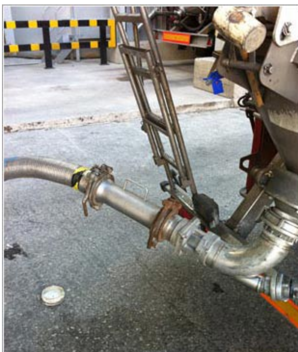
Left: The tanker magnet is shown in situ in the tanker line blowing flour.
