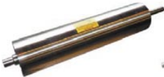
Ferrite head roller for a MRF plant. Face width 1555 x 218mm dia. Crowned face. Shafts machined to order
